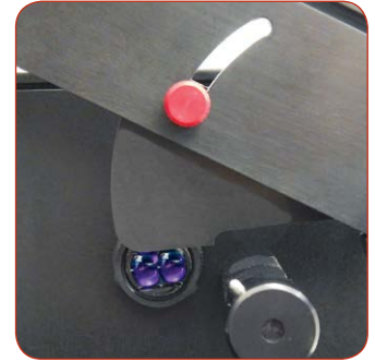
Optical shut-off sensor with adjustable stop
